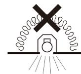
Luminaire not suitable for covering with thermally insulating material
